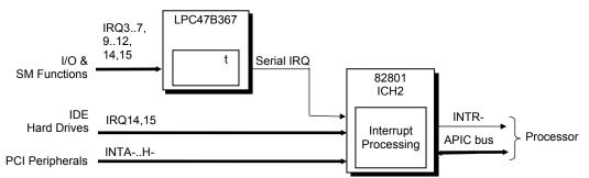
Figure 4-9. Maskable Interrupt Processing, Block Diagram
